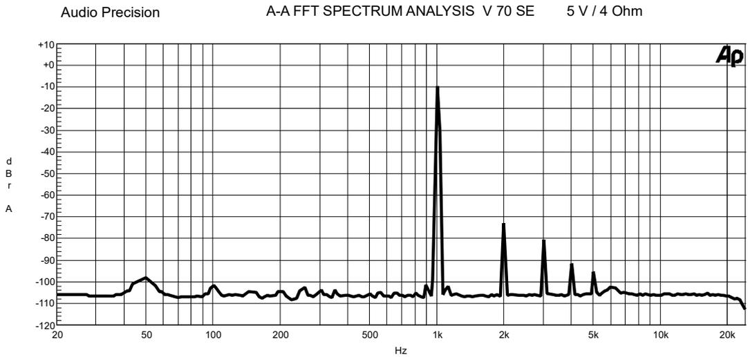
Noise spectrum at 1 kHz / 5 W into 4 ohms – there is no mains interference to be seen. (50 Hz < 200  $\mu$ V, 100 Hz < 70  $\mu$ V) The k2, k3, k4 and k5 noise spectrum is extremely low and falls quickly.
