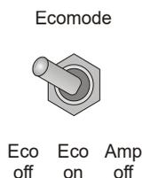
**Eco off:** The Ecomode electronic is off, the amplifier is on.
