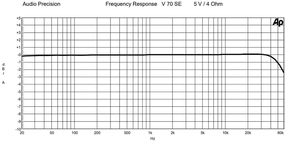
The frequency response curve clearly shows the low frequency extension of the V 70 SE linear to 10 Hz The loss at 20 Hz is less than 0,2 dB.
